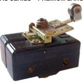
The MICRO SWITCH<sup>TM</sup> 6AS Series consists of two large premium BZ/BA/BM/BE snapaction switches ganged together and actuated by a single actuator. Operating characteristics are dependent upon the type of individual switches and actuators chosen. Field adjustable operating point on one or both basic switches.
